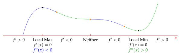
**Definition.** A curve y = f(x) has an inflection point at x = c if the curve is continuous at c and changes from concave upward to concave downward at c (or vice versa).
