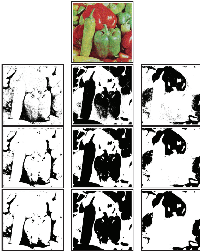
Figure 17. Classifying a real image into three groups. The first row shows the original color image. The second row shows the classification using the original EM algorithm. We plot our classification without feedback (third row) and with one feedback (fourth row).
