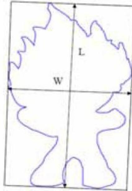
Fig. 3. Minimum bounding rectangle and corresponding parameters for elongation
