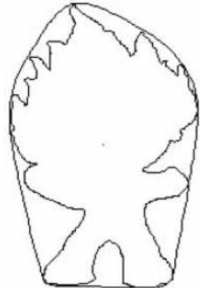
Illustration of convex hull
