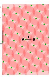
Consider a lattice  $\Lambda$ , and add noise to each lattice point until the entire space is covered. Increase the noise until the space is uniformly covered.
