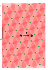
Consider a lattice  $\Lambda$ , and add noise to each lattice point until the entire space is covered. Increase the noise until the space is uniformly covered.
