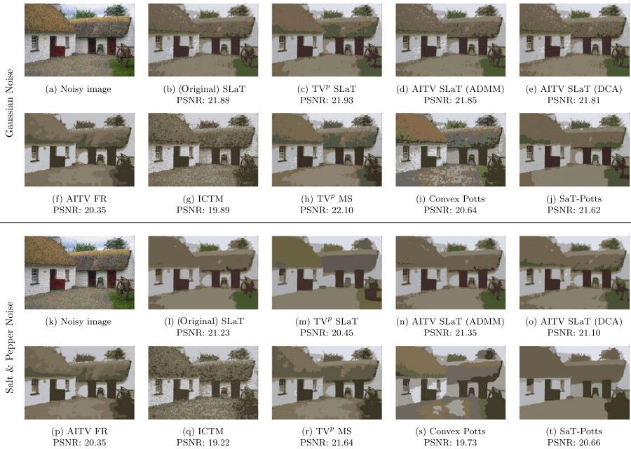
Fig. 14 Segmentation results into k = 6 regions of Fig. 11c corrupted by either Gaussian noise of mean zero and variance 0.025 or 10% SP noise
