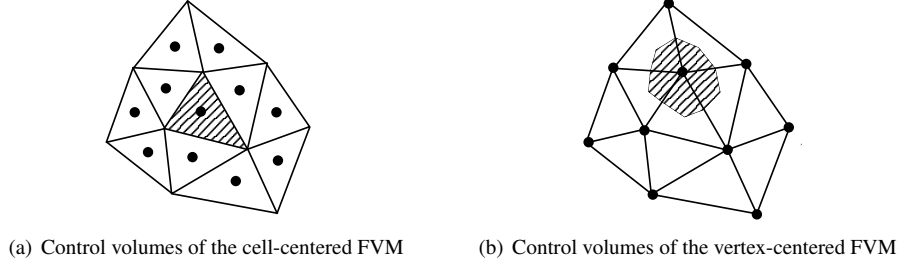
FIGURE 1. Meshes and control volumes of two FVMs. The unknowns are associated to black nodes.
