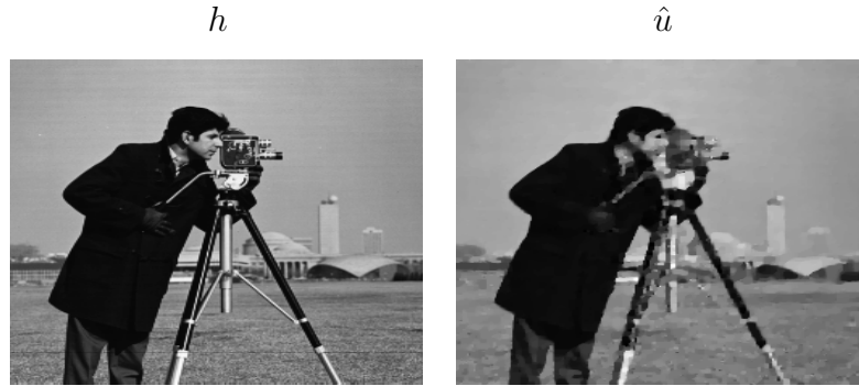
Figure 2.3: Constrained TV minimization of 256 \times 256 cameraman image given 1% of its translation invariant Haar wavelet coefficients
