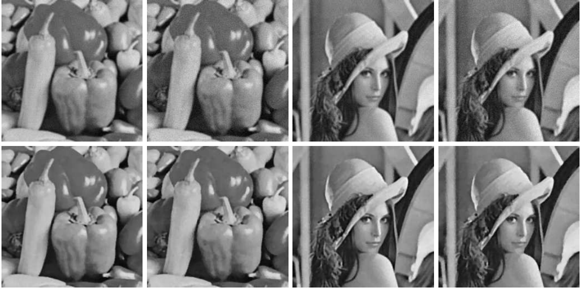
Figure 4.3. Top Row - Noisy blurred images with 5 \times 5 out-of-focus blur of type IV and noise levels \sigma = 5 (left two), \sigma = 8 (right two), Bottom Row - Recovered images corresponding to the above images.
