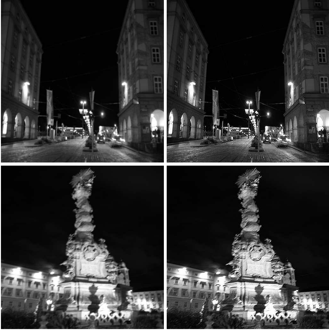
Figure 4.22. Blind deconvolution of night scenes, size reduced to 512 \times 512 . Recovered with a simple guess of a radially symmetric blurring kernel.
