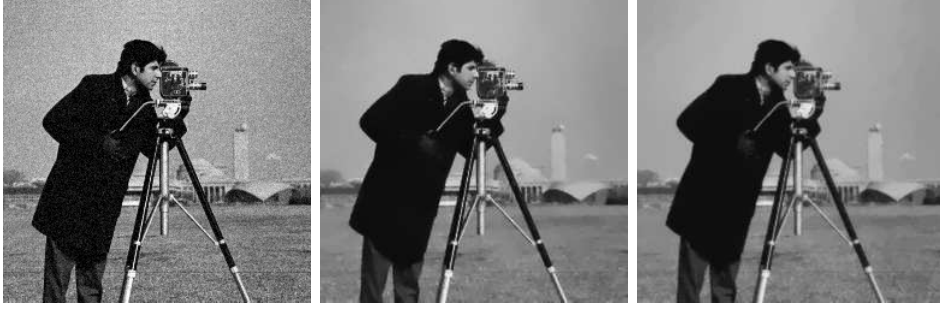
Figure 4.12. Noise level is \sigma = 10 . Best denoising results with p = 1.05 and p = 2 , respectively.
