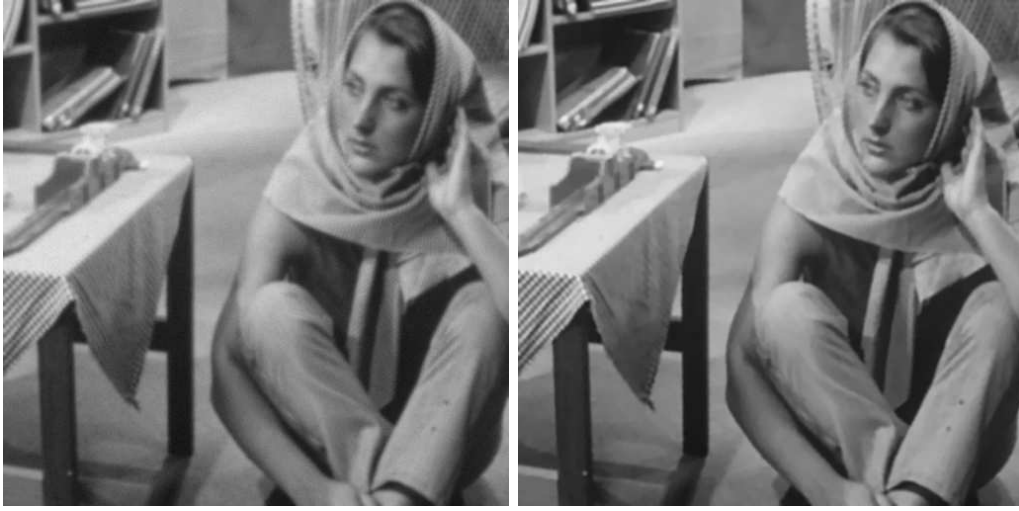
Figure 4.4. Recovery from a noisy blurred image of size 512 \times 512 with 15 \times 15 Gaussian blur of type VI and noise \sigma = 3 . Left: Noisy blurred image, right: Recovered image
