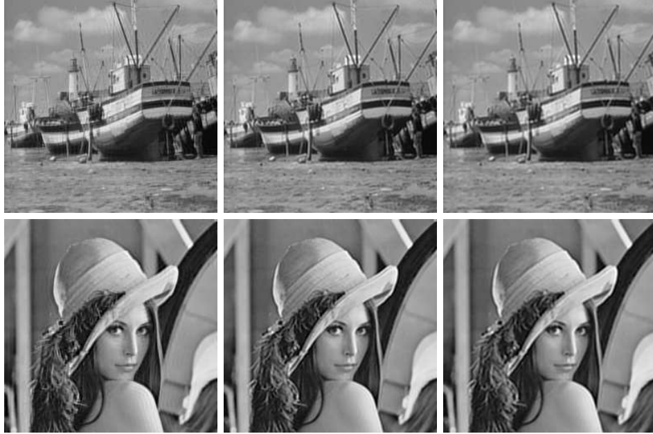
Figure 4.21. Comparison between the three blur types, II and V and VI after 300 iterations. Left (type II): PSNR=32.49 (boat) and 31.98 (woman); middle (type V): PSNR=31.54 (boat) and 32.60 (woman); right (type VI): PSNR=29.85 (boat) and 31.05 (woman).
