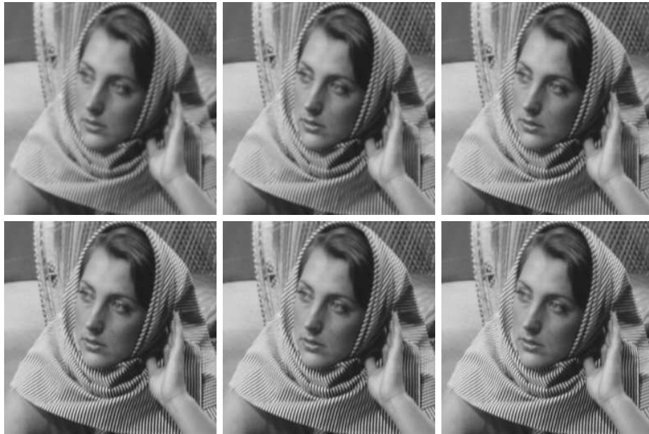
Figure 4.16. 3 \times 3 average kernel, blur type I; Left to Right and Top to Bottom: Blurry image, Recovered image with p = 2 , p = 1.9 , p = 1.01 , p = 1 , Original image.
