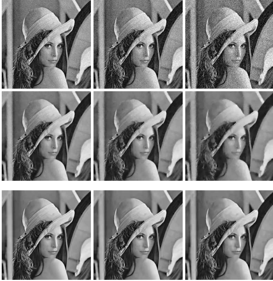
Figure 4.14. \delta = 0.2, p = 1.1, dt = 0.007 ; top row, from left to right: Noisy images with \sigma = 10, 15, 25 , middle row: Images recovered from the noisy images right above, bottom row: Images recovered with a state-of-the-art denoising algorithm, BM3D [4], for comparison.
