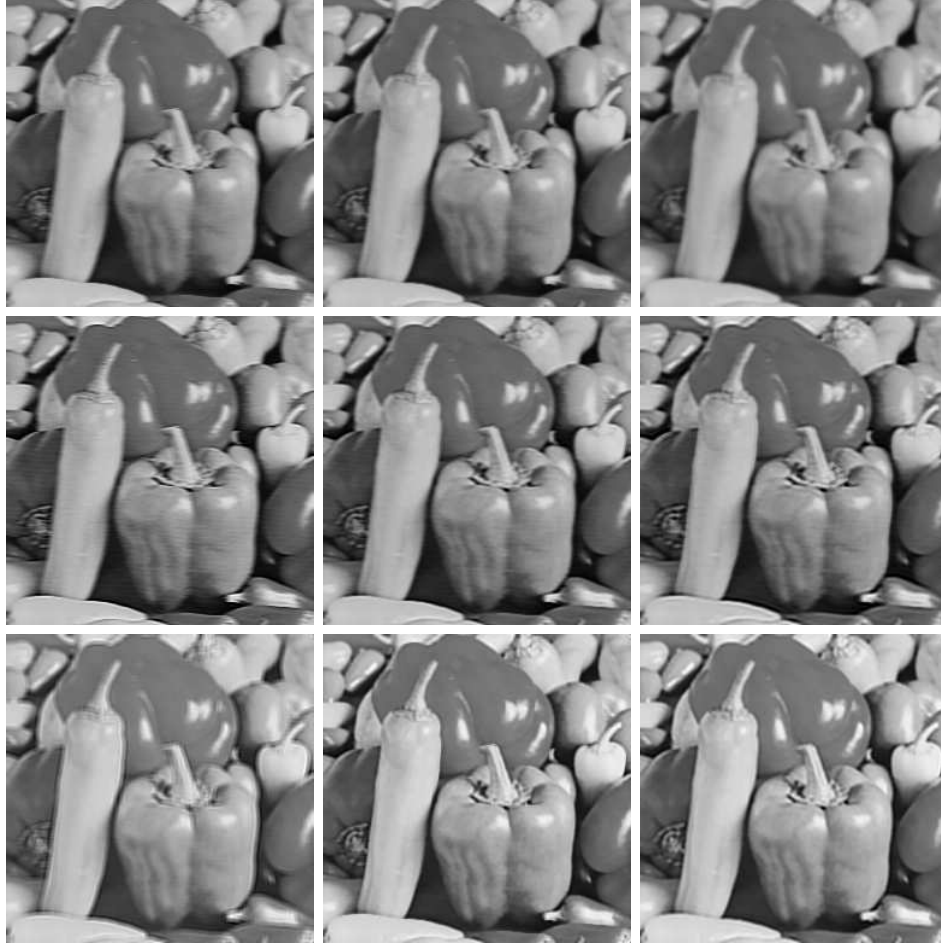
Figure 4.23. Recovery results. Top row : Blurry images, Middle row : Recovered images by our proposed model, Bottom row : Recovered images by the ROF model. Left column - 1 \times 5 horizontal motion blur, Middle column - 3 \times 5 blurring kernel A in Table 4.7, Right column - 3 \times 5 blurring kernel B in Table 4.7.
