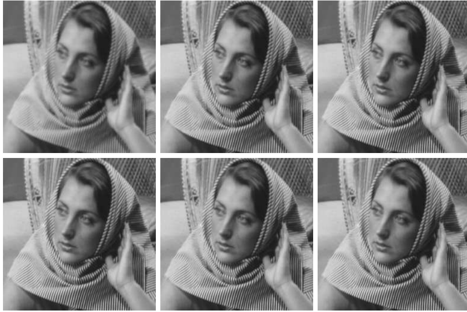
Figure 4.17. A closer look at the case p = 1.01 in Table 4.6. First row, from left to right : Blurry image, output images after 10 and 20 iterations (PSNR values : 26.49, 31.20, 32.91); second row, from left to right: output image after 30, 40, and 50 iterations (PSNR values : 33.76, 34.30, 34.72). Computational time for 10 iterations amount to approximately 3.6s.
