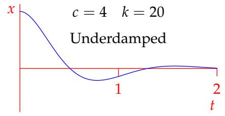
**Sports car** suspensions are typically closer to *critical damping*:  $c$  and  $k$  are very large, and  $c^2 \approx 4km$  for a fast, stiff ride. Sports cars ride low to the ground for aerodynamics and so cannot bounce around. Tires also need to quickly be forced back to the road after going over a bump lest the vehicle lose grip and crash.
