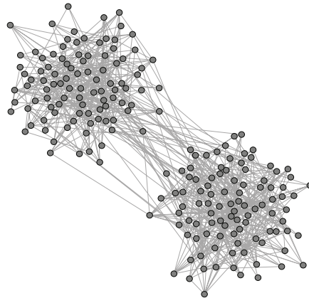
Figure 2.3.3. A network generated according to the stochastic block model G(n, p, q) with n = 200 nodes and connection probabilities p = 1/20 and q = 1/200 .
